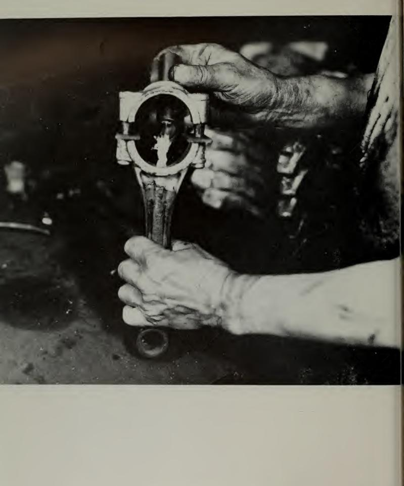
Any oil holes appearing in various places on the cap or the bearing end of the rod (varying with the type of rod) are plugged with asbestos wicking as shown above. In some instances small cork stoppers are used and even toothpicks on the smaller rods. This caulking process prevents the babbitt from plugging up the oil holes.
